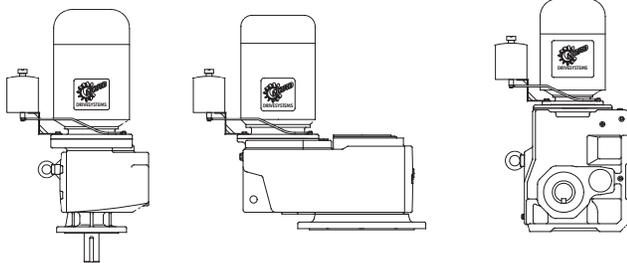
4. Be sure to use the proper fittings. Assemble one end of the vent-hose assembly (21) to bottom of the chamber and one-end to the reducer.
