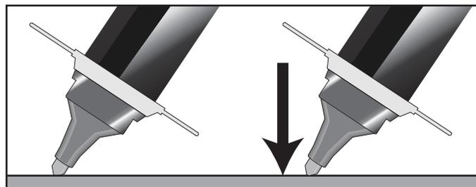
Press the pen tip down on the surface until solution fills the pen tip. Apply the sealer pen solution to the metal surface with firm, smooth, even strokes, covering all of the edges. Overlap each stroke and allow to dry.
