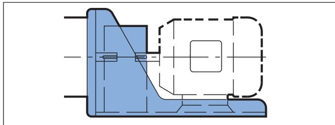
Each scoop bracket includes the coupling for the motor and the coupling guard.
