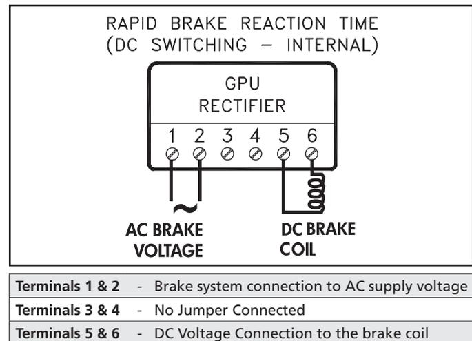
The DC-switching function of the GPU brake rectifier can be disabled (and AC-switching can be enabled) by shorting terminals 3 & 4 via a jumper or an external switch.
