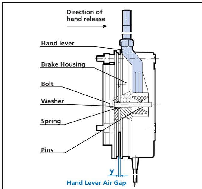
1. Place the hand-lever over the brake housing (as shown) and align the pins.
