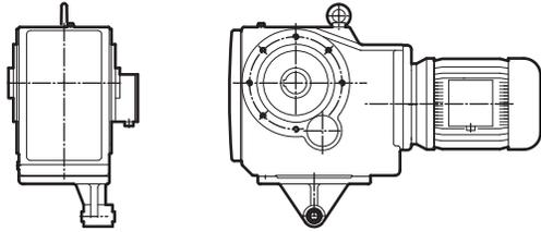
Torque Arm (K) with rubber buffer
