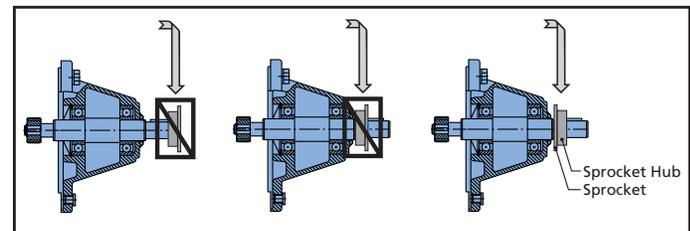
Align the driver sheave or sprocket with the driven sheave or sprocket by placing a straight-edge length-wise across the face of the sheaves or sprockets. Alignment of bushed sheaves and sprockets should be checked only after bushings have been tightened. Check horizontal shaft alignment by placing one leg of a square or a level vertically against the face of the sheave or sprocket.
