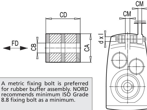
A metric fixing bolt is preferred for rubber buffer assembly. NORD recommends minimum ISO Grade 8.8 fixing bolt as a minimum.
