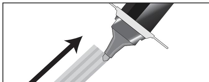
Frequent short jabs to re wet the application rip are preferred to maintain constant coating weights and avoid over-wetting the felt tip.
