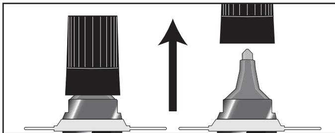
To activate, hold the Touch-N-Prep® pen upright and pop off the cap. Do not twist or turn to remove the cap, since this may result in the pen leaking. Hold the pen tip down onto a clean surface to begin the flow of solution to the tip.
