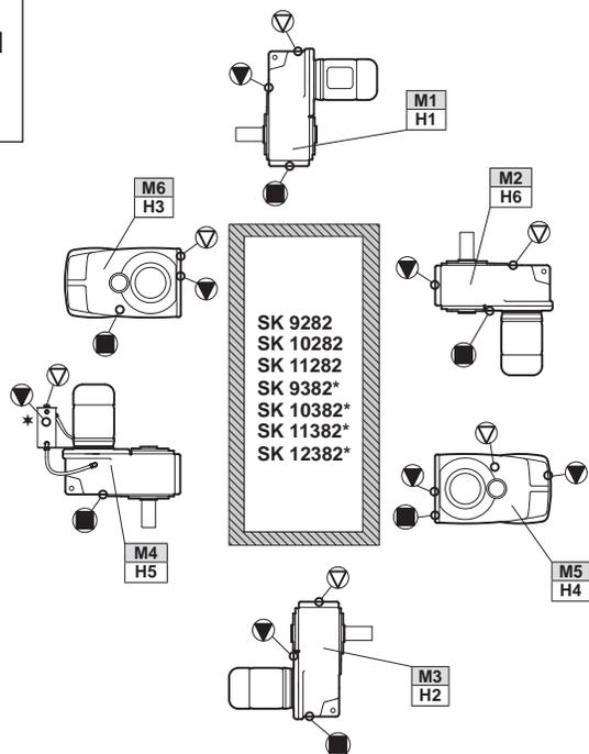
\* Oil level for 3 stage gear units
