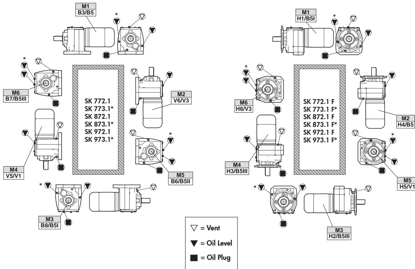
\* Oil fill level for three stage gear units.
