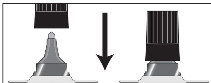
Always immediately replace the cap when not in use to avoid evaporation and contamination.
