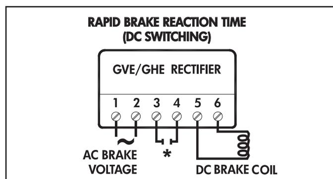
Terminals 1 & 2 - Brake system connection to AC supply voltage
