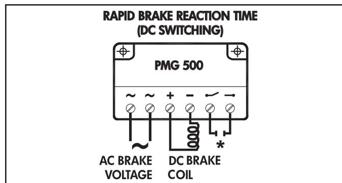
Terminals ~ & ~ - Brake system connection to AC supply voltage
