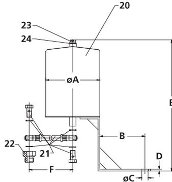
1. Secure the gear reducer in the proper mounting position for the application and remove the vent plug from the gear reducer. The hose assembly kit (21) will be fitted to the reducer using the housing port provided.
