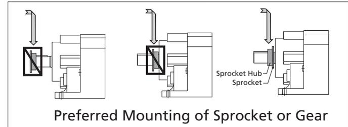
Align the driver sheave or sprocket with the driven sheave or sprocket by placing a straight-edge length-wise across the face of the sheaves or sprockets. Alignment of bushed sheaves and sprockets should be checked only after bushings have been tightened. Check horizontal shaft alignment by placing one leg of a square or a level vertically against the face of the sheave or sprocket.
