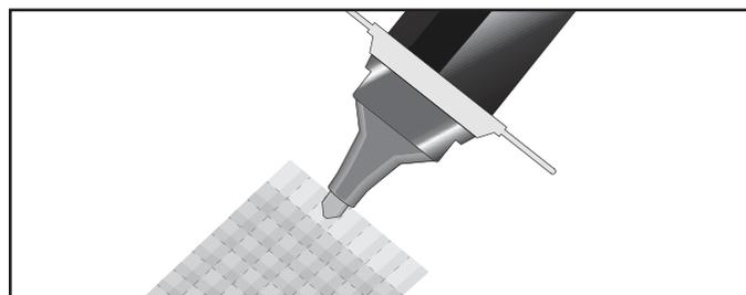
Within 5 minutes of the first coat, apply a second coat at a 90° angle to the first coat with the same smooth, firm stroke.
