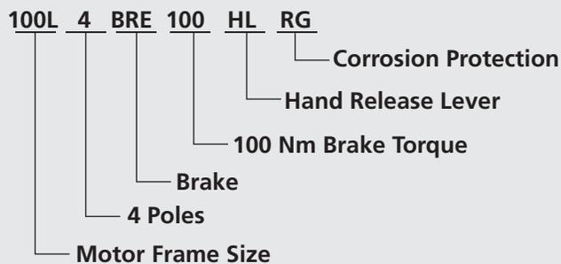
100 Frame Motor with 4 poles, Brake, 100 Nm with a hand release lever, corrosion protected brake, and a current sensing relay.
