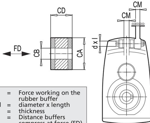
**FD** = Force working on the rubber buffer
