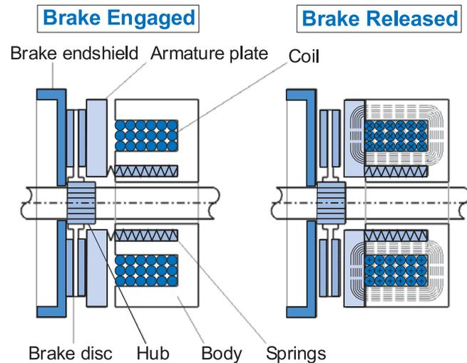
NORD brakes are DC voltage brakes and in most instances are supplied with a motor mounted brake rectifier for easy connections to AC power. AC power is taken directly from the power line or from the terminal block of the motor and converted to DC by the supplied rectifier.
