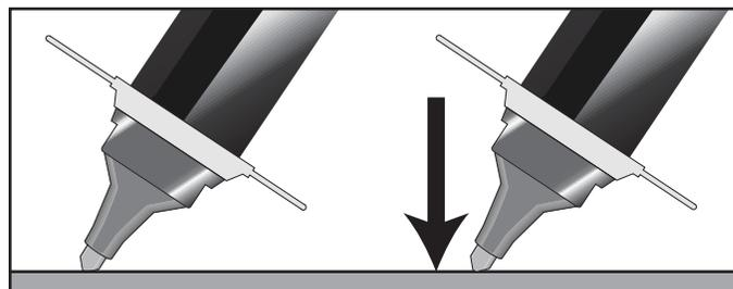
Press the pen tip down on the surface until solution fills the pen tip. Apply the Alodine® 871™ solution to the metal surface with firm, smooth, even strokes, covering all of the edges. Overlap each stroke and allow to dry.
