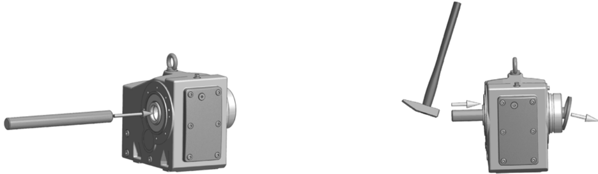
Figure 5: Removing the factory-fitted closing cap
