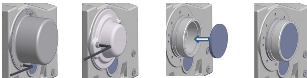
Figure 13: Fitting the covers, Option SH, Option H, and Option H66
