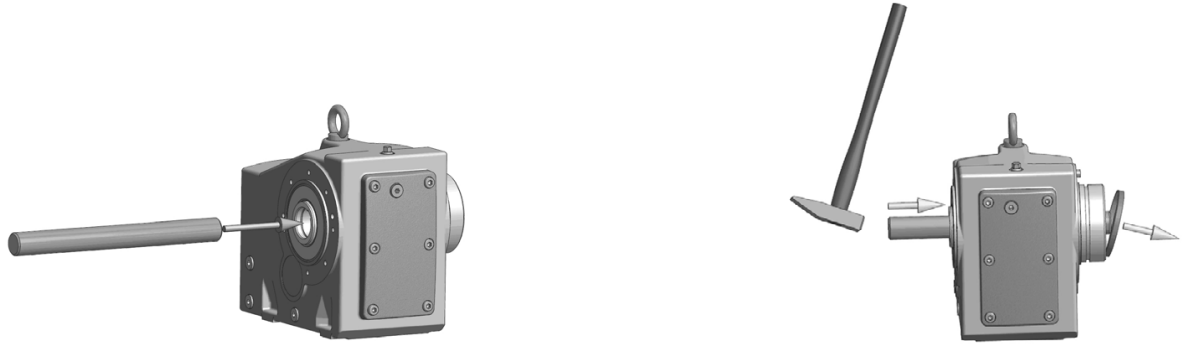
Figure 5: Removing the factory-fitted closing cap
